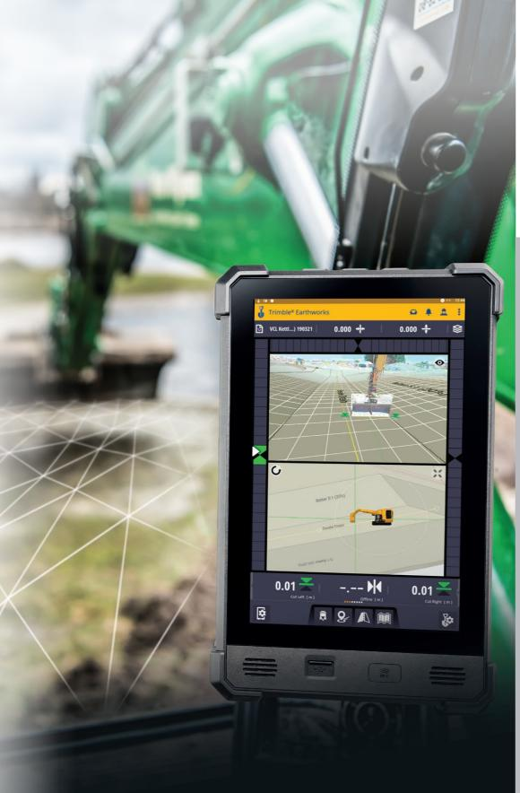
**2D CONFIGURATION FOR HEIGHT AND SLOPE** - Flexible starter solution for excavation, canal and trench construction, grading and profile work—the start of productivity.
