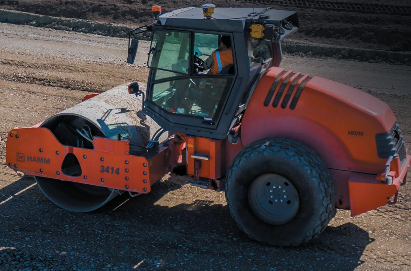
Trimble Earthworks supports 4-drum landfill compactors. The Landfill Compaction Algorithm (LCA) gives operators the ability to configure multiple compaction parameters. It helps avoid unnecessary passes that waste time and fuel, and alleviates thick layer material placement that leads to insufficient compaction. LCA allows contractors to customise the system to the characteristics of the site, allowing users to define their own best practices for a more efficient landfill operation.
