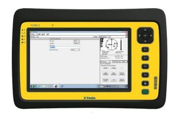
Released in 2012, the YUMA 2 has an internal 3G modem that won't be able to connect to the internet after the shutdown even with a SIM card. This will mostly affect GNSS surveys using VRS services or Trimble Connect data workflows (or other remote data transfer solutions). The shutdown does **not** affect the connection between the instrument and controller, just the downloading of position correction information and internet connectivity.
